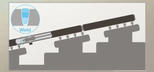
**6** The prepared double-joints are now joined to the end of the pipeline in a semi-automatic welding process Qualified welders oversee each of the steps to ensure that welding procedures meet Nord Stream's and authority approved quality standards.
