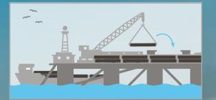
**1** The pipes are unloaded from the pipe carrier vessels and stacked on the storage areas on each side of the laybarge. Pipes are delivered regularly to ensure that the are always enough supplies on board to maintain the 24-hour construction schedule.
