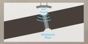
**7** The weld of the double-joint that has been welded onto the main pipeline also undergoes ultrasonic testing at another non-destructive testing station. Any unacceptable flaws will be repaired, and the weld rescanned so that it meets international quality standards.
