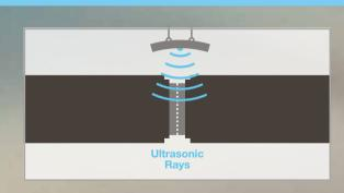
**4** The double-joint is moved to the non-destructive testing station where every millimetre of the weld undergoe ultrasonic testing to detect any unacceptable flaws. If required, the defect will be repaired and the weld rescanned to meet international quality standards.
