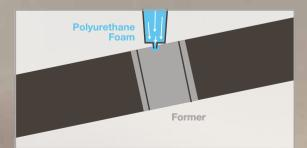
8 Once the weld is confirmed acceptable, a corrosion-resistant, heat-shrink sleeve is applied around its entire circumference. Then, polyurethane foam is poured into a mould surrounding the weld area. This foam hardens, providing further protection.
