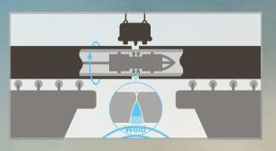
**3** At the double-joint welding station, two bevelled, 12-metre pipe joints are aligned and welded together to create a double-joint segment measuring 24 metres These double-joint sections will later be connected to the main pipe string.
